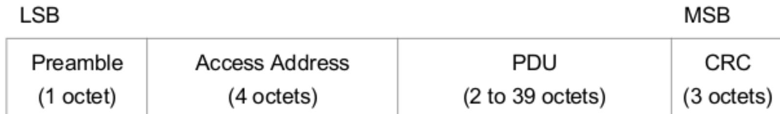
*Figure 2.1: Link Layer packet format*
