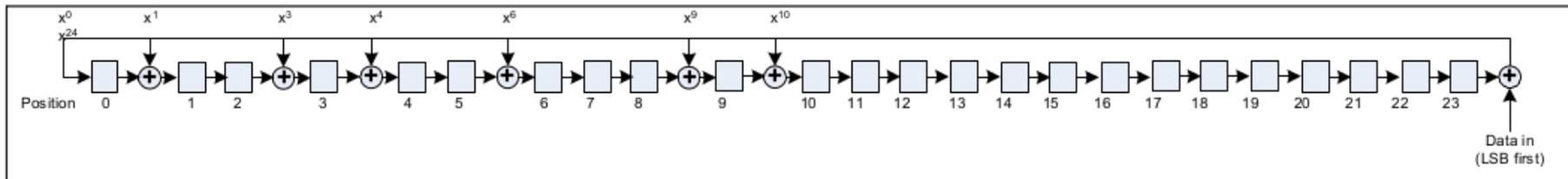
Figure 3.2: The LFSR circuit generating the CRC
