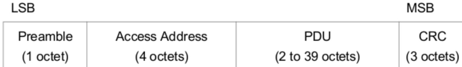
*Figure 2.1: Link Layer packet format*
