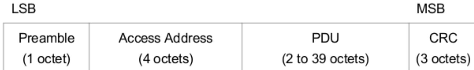
Figure 2.1: Link Layer packet format
